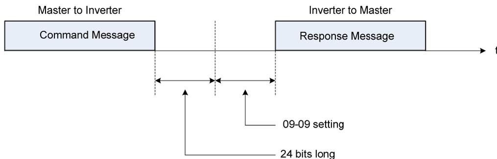
**Figure 4.4.67 Communication Message Timing**
