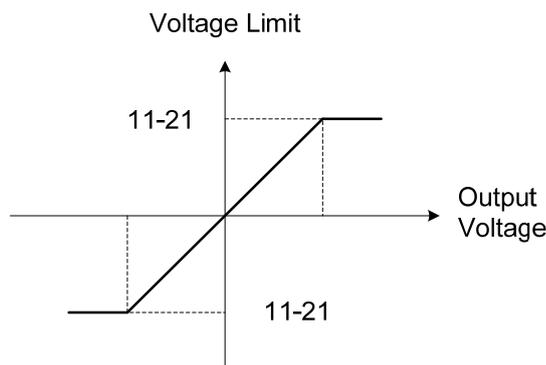
Figure 4.4.80 Voltage limit value of commissioning operation
