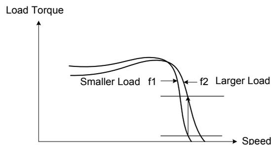
**Figure 4.4.90 Slip compensation output frequency**
