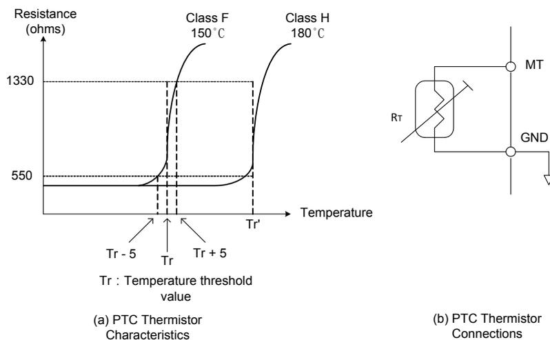
**Figure 4.4.66 Protection of motor overheating**
