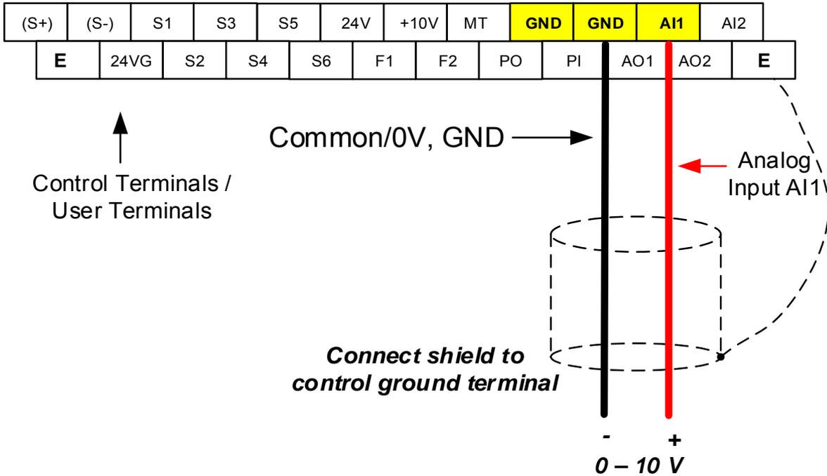
Analog Reference: Potentiometer / Speed Pot (Setting 00-05 = 1)
