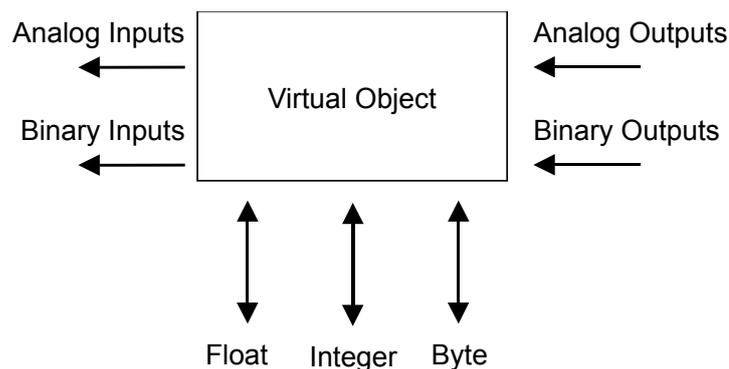
The object of N2 Slave has grouping and every group data can set the address of 0-255, abbreviated for NPA (Network Point Address).
