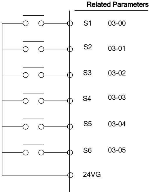
Figure 4.4.13 Multi-function digital input and related parameters
