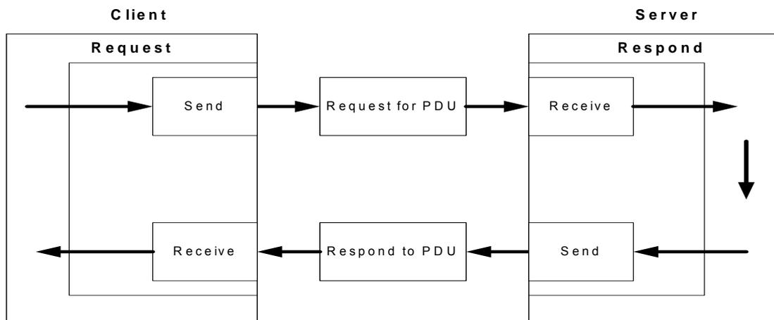
All BACnet devices have the application programs to manage the requirements of device motion and executing services. Take work station for example, the application program needs to keep the display value of every input so it requires sending the service request to the object of other device to update the display value of input. The application program of the device needs to respond to the service requirements. Refer to the following figure.
