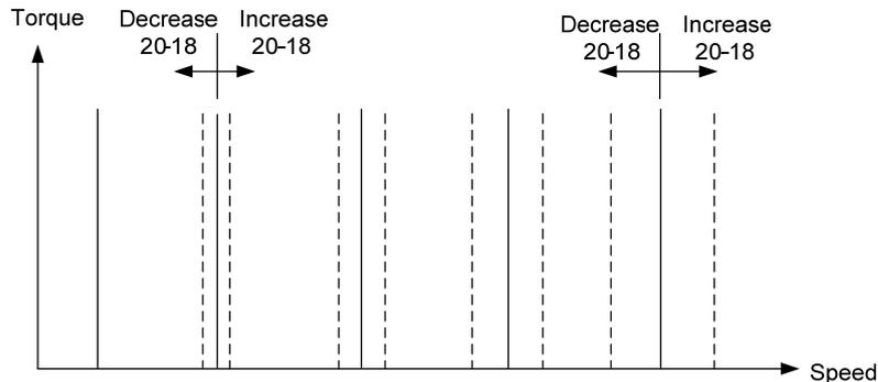
**Figure 4.4.100 Effect on the torque-speed curve from 20-17**
