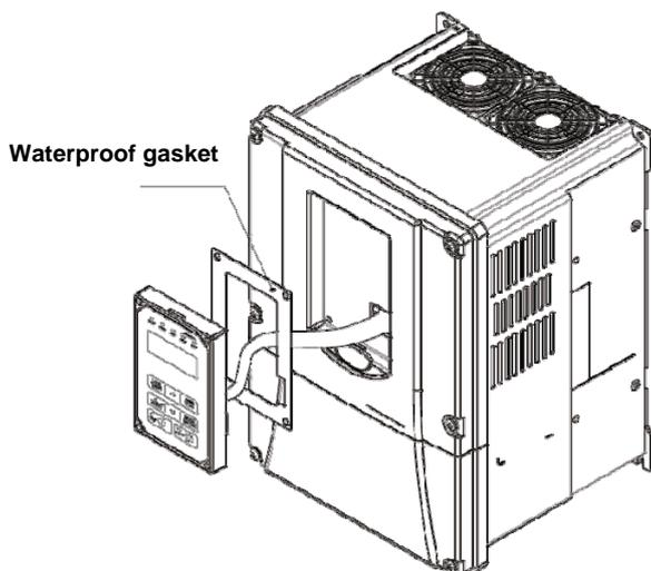
**Step 3:** Pull out operator and remove power line
