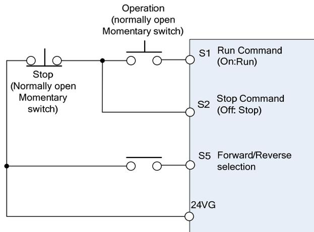
**Figure 4.4.2 Wiring example of 3-wire**
