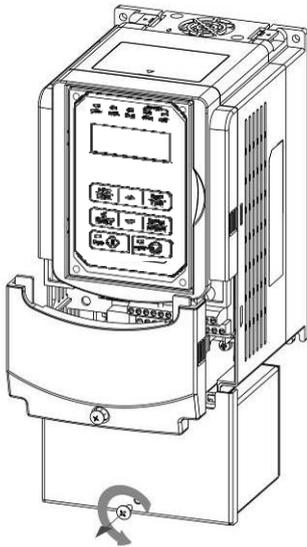
**Step 3:** Unscrew filter section
