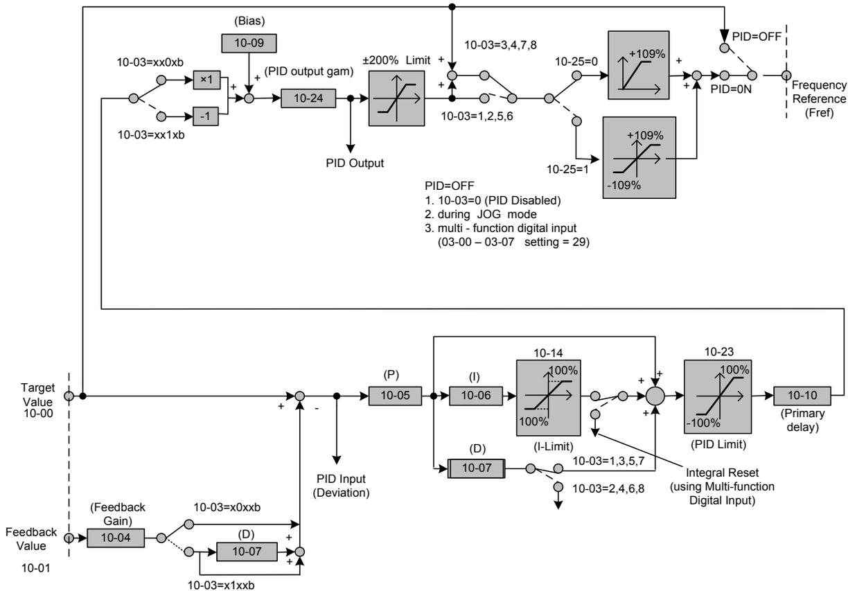
The amplitude of the error can be adjusted with the Proportional Gain parameter 10-05 and is directly related to the output of the PID controller, so the larger the gain the larger the output correction.
