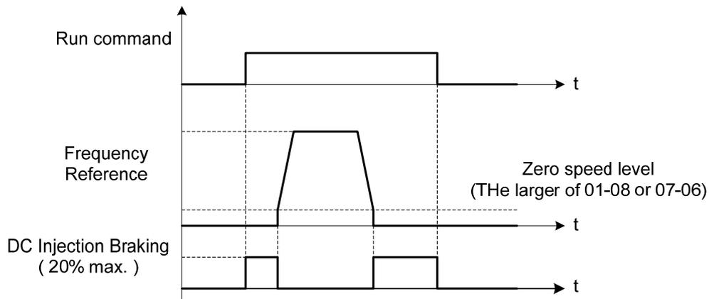
Figure 4.4.84 Zero-speed braking operation
