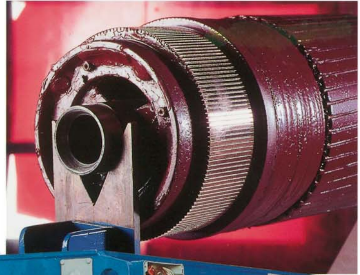
Rewinding with reconstitution of collector Rotor of mandril motor.
