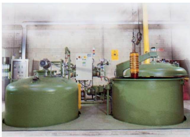
Plant for impregnation with resin under vacuum, capacity 9 cubic metres
