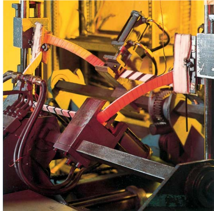
Shaping coils for M.T. motors
